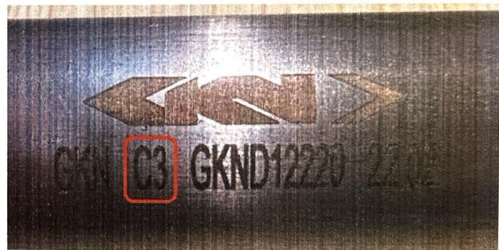
CV joints: Laser Marking GKN + Chevron + Plant Code **C3** + Part Number.
